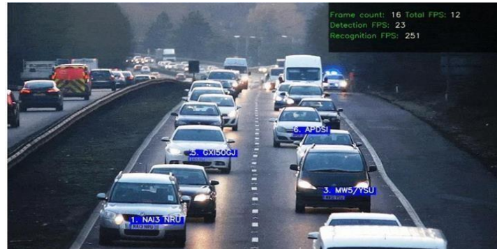
Figure 1: Figure 1: Automatic (Machine Language) License Plate Recognition System- Computer algorithms process these images to find and identify the characters on the license plates. Here's a simplified explanation of how it works:
